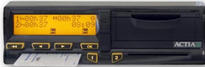
Printouts can only be made if the vehicle ignition is switched on.
