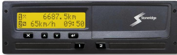
Printouts can only be made if the vehicle ignition is switched on. **Printouts produced by the Stoneridge SE50 Digital Tachograph Vehicle Unit ALWAYS show UTC time.**
