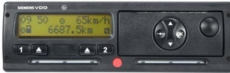
Printouts can only be made if the vehicle ignition is switched on. **Printouts produced by the Siemens DTCO 1381 Digital Tachograph Vehicle Unit ALWAYS show UTC time.**
